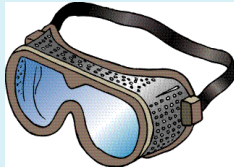
(Goggles with direct vents are not suitable for protection from chemical splattering or smoke)
